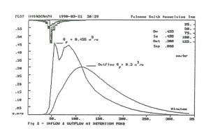
Data regud: For a user-specified peak outflow, MIDUSS computes the required storage volume. The user may then adjust a table of Depth-Discharge-Volume relations to describe the characteristics of the reservoir and the outflow structure. The maximum and penultimate stages are computed by MIDUSS; if only 3 stages are used no further data is required from the user. The user may optionally reduce the routing time-step to a submultiple of the runoff time increment dT.
